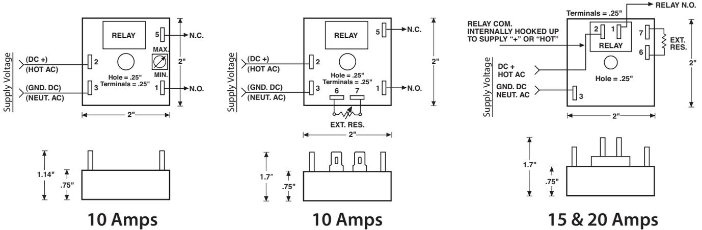
**Input Voltage:** VDC: 12, 24-28, or 48
